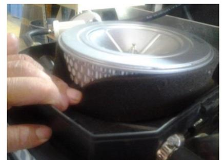
HONDA engine area. Cellulose, fiberglass, or stonewool entering the engine cooling fan will gather over time and limit the engine's effectiveness in cooling itself.
