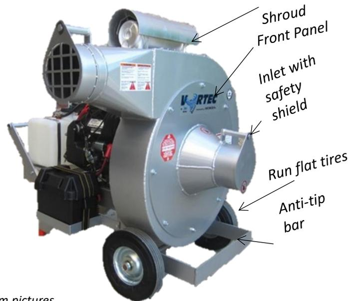
**Inlet:** The inlet diameter is 6 inches.
