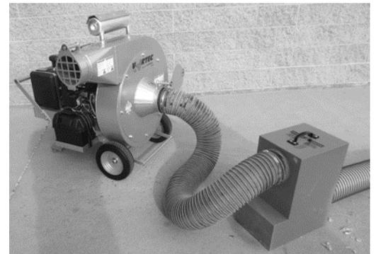
5. Attach hose or vacuum bag to the machine's outlet using a hose clamp.
